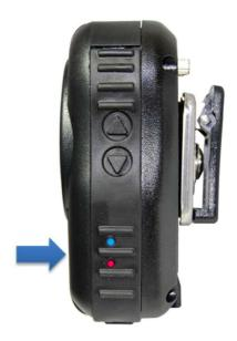
2. When you see LED flashing in a pattern of RED-BLUE-RED-BLUE, BTH-600 is in pairing mode.
