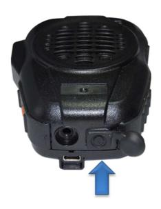
1. Press and keep holding the power switch for 6 second from cold start
